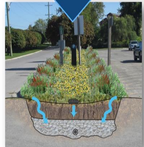
Example of a bioretention retrofit of a median in a parking lot, Port Perry
