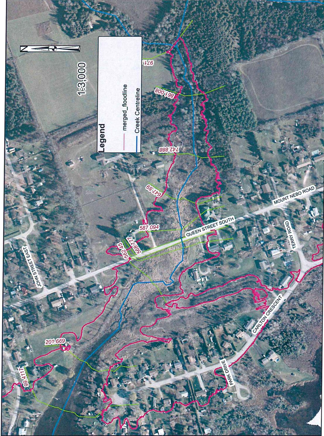
Figure 8.8 Comparing Pigeon River Dam Pond, Creek, and Regulatory Flooding Extents
