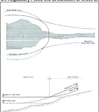
Figure 8.4 Regulatory Flood line at Junction of Creek and Lake
