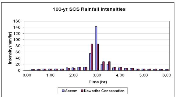
The worst case storm (the duration and distribution producing the highest discharges at key nodes) is selected as the critical event for the watershed. Detailed rainfall information is shown in **Appendix C**.
