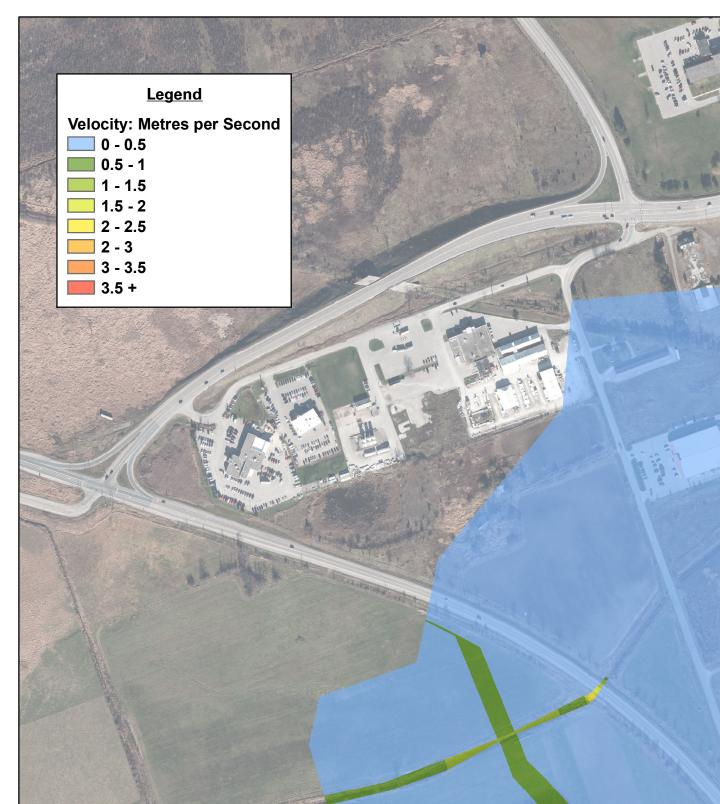
Figure 13.5: Flood Velocities in Commercial Area - Timmins Dynamic Storm 1 centimetre = 45 metres
